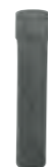
Aluminum 15ml Sleeve GLB-15A-FA Sleeve bore (ΦxL) :18 x 90 Radius (mm) :116 Max.RPM : 4,000 Max.RCF (g-force) : 2,075
