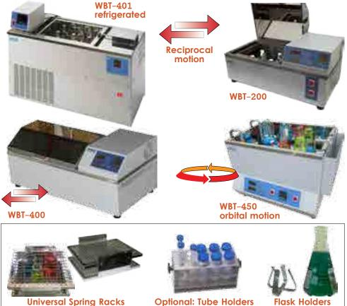
These reciprocating water bath shakers are available in three models. Model WBT-200 small platform 250x300mm, Model WBT-400 large platform 300x400mm & Model WBT-401 refrigerated to 0°C. Temperature control is precise, temp. range of 5°C above ambient to 100°C, speed range 20 - 200 rpm, heat loss and evaporation minimized with use of stainless steel hood cover.
