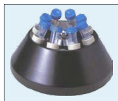
RA-1508 15ml x 8pcs Max. 5,500rpm
