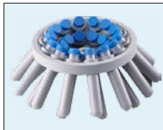
AR-1524 5-15ml x 24pcs Max. 4,000rpm
