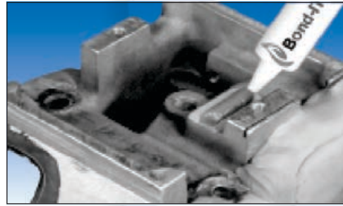
Bond-IT 7056AL Fills a Casting Before Re-Machining
