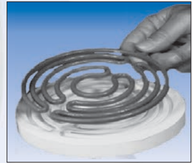
Placing Heater Coils in Insulating Disk
