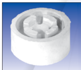
Replicast Mold Ready For Casting
