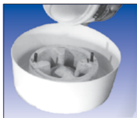
Pouring Replicast Around a Model
