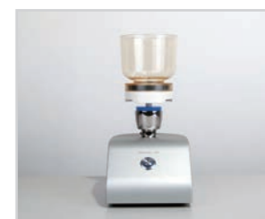
WaterVac 100 with Magnetic filter holder
