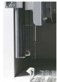
Sample/Reagent Probe with Liquid Level Detection.
