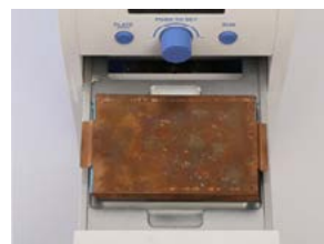
Step.3-2 Put the weighted sealing flake if the film is curly
