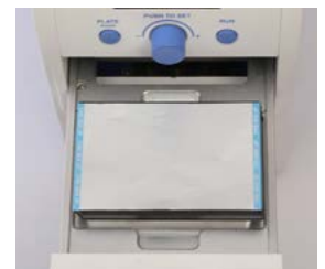
Step.3-1 Put a sealing film
