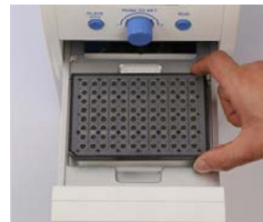
Step.2 Put the adapter, plate
