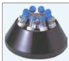
RA-1508 15ml x8pcs Max. 6,000rpm
