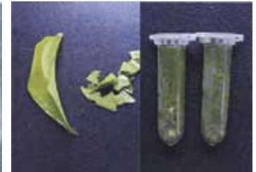
Leaves: Micro vial adapter plate/Micro vials/3mm tungsten carbide bead per vial. Completely homogenized.
