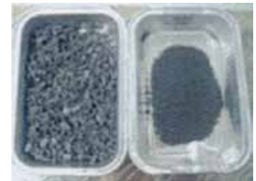
Rubber: 50ml steel jar/20 mm steel Ban after cryogenic grinding.
