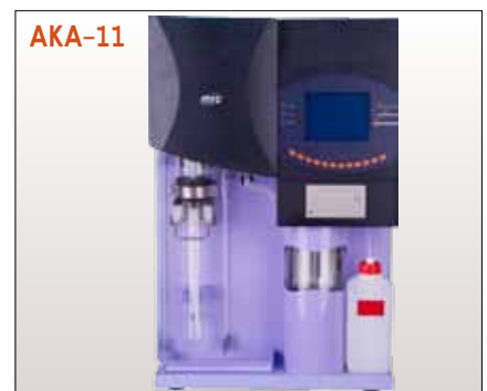
AKA-11 Automatic Kjeldahl Analyzer Page 4
