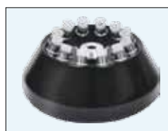
RA-1512HS 15ml x 12pcs Max. 9,000rpm
