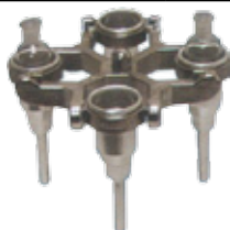
RS-50 25ml x 4pcs Max. 1,200rpm
