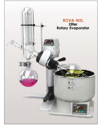
The equipment for purification distillation test rotates and shapes a thin film in negative pressure condition by heating, evaporates efficiently, and then condenses and recollects solvent to purify and separate. The products can be made into system devices with Multi-purpose Circulating Water Vacuum Pump, Diaphragm Vacuum Pump, Low Temperature Circulating (vacuum) Pump, Circulating Cooler, Constant Temperature Ccirculator, Low Temperature Ccooling Lliquid Circulating Pump.
